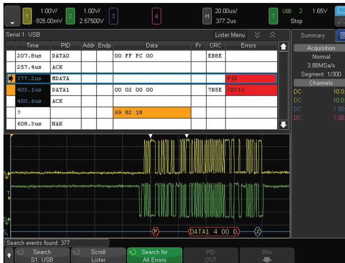
Figure 21. USB 2.0 trigger, decode and "lister" display.
