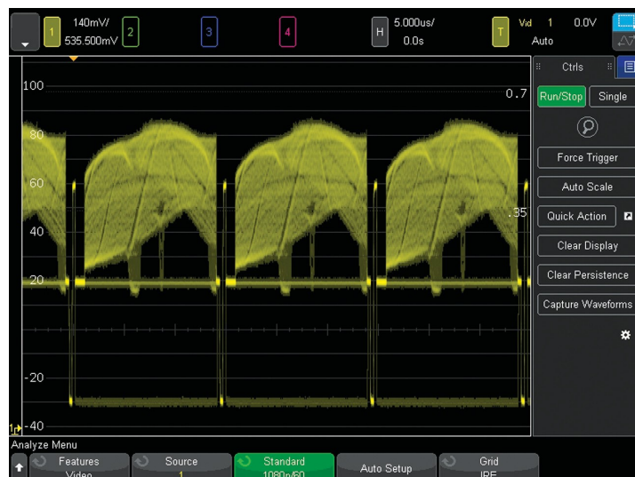
Figure 27. Triggering on 1080p HDTV signal analysis.
